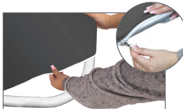
Step 5: Finally, pull the banner down tightly. This step requires some assistance. So ask a friend if they can connect the zipper and begin closing the zipper, while you maintain tension on the banner.
